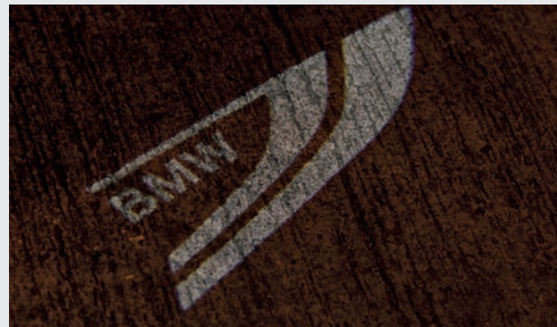
The Lights Package also includes a welcome greeting. When the vehicle is unlocked, an LED light source in the driver's-side exterior mirror projects onto the ground.
