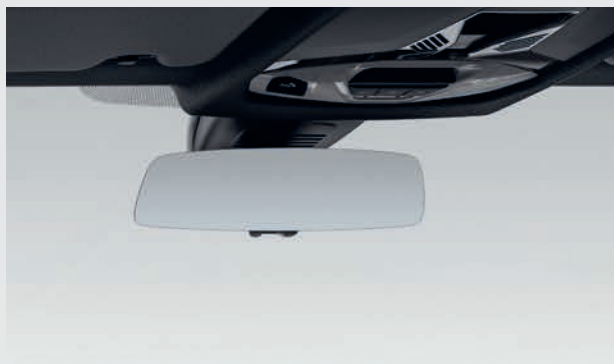
The Frameless Interior Mirror , with electromagnetic coating, consists of automatic anti-dazzle function via integrated sensors that measure light incident from behind and automatically dim the interior mirror if the measured light intensity is high enough to cause dazzling.
