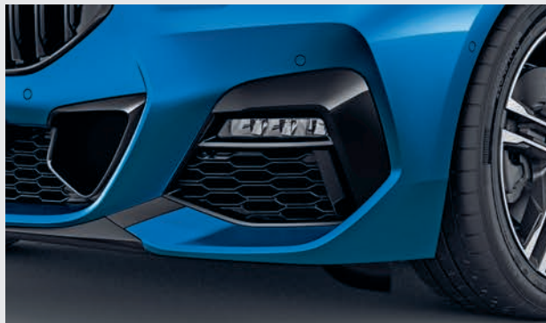
LED Fog Lights increase short-range visibility in fog or precipitation, improving night-time driving safety.
