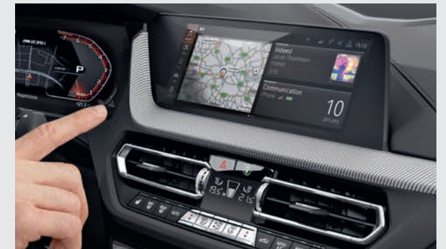
With BMW Gesture Control , selected functions can be operated by means of defined hand movements. Simple gestures such as 'swiping' or 'pointing' are identified in the recognition area above the centre console and trigger functions such as accepting or rejecting an incoming telephone call, proceeding or cancelling navigation as well as starting and ending voice recordings.
