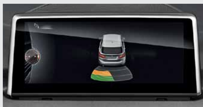
The Park Distance Control (PDC) with Rear View Camera allows for easy parking and manoeuvring in confined spaces. Acoustic signals and a visual indicator in the Control Display tell you when the rear of the vehicle is approaching an object. Distances are measured by ultrasound sensors in the bumper.
