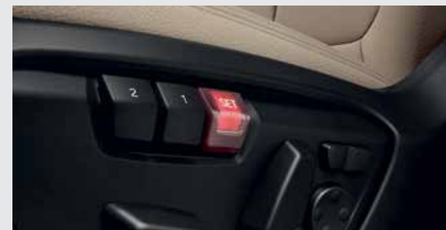
The Electric Seat Adjustment is easy to use and the memory function allows users to save their preferred settings for the seat and exterior mirrors.
