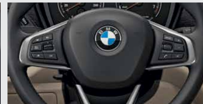
The Multifunction Steering Wheel can be used to operate the telephone, voice control and audio functions via the buttons on the steering wheel. The Manual Speed Limiter is also integrated. For example, it can be used to set an upper limit of 50 km/h for city driving.
