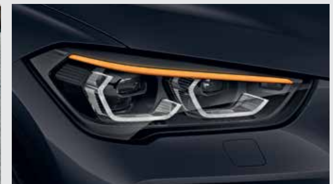
LED Headlights with low-beam and high-beam headlights include LED turn indicators.
