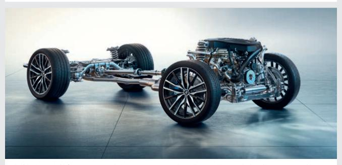
The Adaptive 2-axle Air Suspension makes driving particularly comfortable with high driving dynamics and makes it easier to get in and out and load the vehicle. The air suspension automatically keeps the vehicle at a constant height regardless of the load. It can also be raised or lowered manually at the touch of a button.
