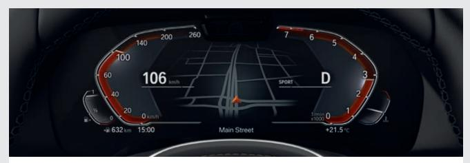
The 31.2 cm (12.3 inches) Multifunctional Instrument Display allows a fully digital display of different content, in addition to speed and revs, including navigation instructions, radio/multimedia track lists and phone lists.
