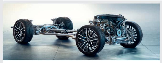
The **Adaptive 2-axle Air Suspension** ensures extremely comfortable driving with great driving dynamics. The air suspension automatically keeps the vehicle at a constant height, regardless of the load. The driver can raise or lower the vehicle in an adjustment range of approx. 80 mm via a toggle switch in the centre console or via BMW Display Key.
