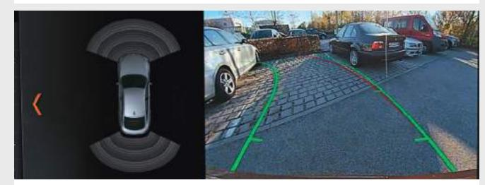
Rear View Camera with Park Assist3 - Camera and ultrasound-based parking assistance system.
