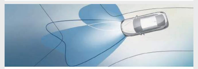
With the **fully adaptive LED headlights,** not only does the outer light move with the steering but also the 4 source LED (low and high beam) including DRL's which distinguishes the look of the BMW X3 both at night and during daytime.
