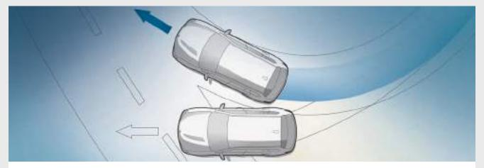
**Dynamic Stability Control (DSC)** permanently assesses the vehicle's movements and stabilises it using engine and braking regulation when unstable driving conditions are detected. Additional features of DSC are, for example, brake drying, braking readiness or the Hill-Start assistant, which holds the vehicle briefly in place when starting on inclines to prevent it from rolling backwards.
