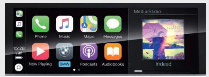
Preparation for Apple CarPlay®<sup>1, 2</sup> supports the convenient and wireless use of selected iPhone® functions in the vehicle. This allows smartphone content and functions such as music, iMessages/text messages, telephony, Siri and selected third-party apps to be displayed and operated via the vehicle's user interface and via voice control.
