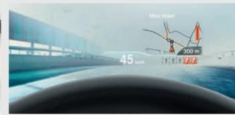
The **BMW Head-Up Display** offers a full-colour projection of driving relevant and situational information onto the windscreen with improved resolution of 800 x 400 pixels.
