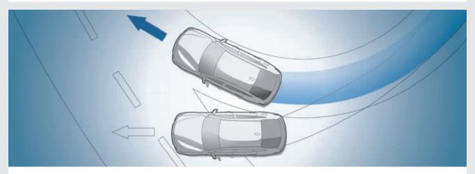
**Dynamic Stability Control (DSC)** permanently assesses the vehicle's movements and stabilises it using engine and braking regulation when unstable driving conditions are detected. Additional features of DSC are, for example, brake drying, braking readiness or the Hill-Start Assistant, which holds the vehicle briefly in place when starting on inclines to prevent it from rolling backwards.
