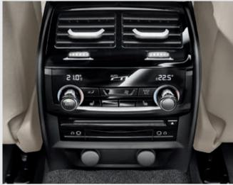
The **Automatic Air Conditioning with Four-Zone Control** comes with the equipment included in automatic air conditioning with two-zone control with extended features, along with two air vents in the B columns. Additionally, the rear passengers can individually adjust their own climate via a separate control element with display.
