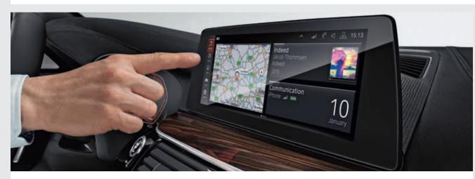
With **BMW Gesture Control**, selected functions can be operated by means of defined hand movements. Simple gestures such as 'swiping' or 'pointing' are identified in the recognition area above the centre console and trigger functions such as accepting or rejecting an incoming telephone call, proceeding or cancelling navigation as well as starting and ending voice recordings.
