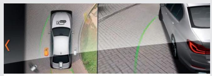
**Parking Assistant with Surround View Camera** makes parking and manoeuvring the vehicle easier. The Parking Assistant with linear guidance parks the vehicle automatically, parallel or perpendicular to the street. Surround View includes the camera-based functions like Rear View Camera, Panorama View, Top View and 3D View. The cameras in the exterior mirrors as well as at the front and rear of the vehicle allow for a 360° all-around view.
