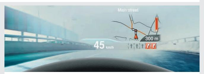
**BMW Head-Up Display** offers a full-colour projection of driving relevant and situational information onto the windscreen with improved resolution of 800 x 400 pixels.
