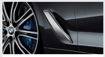
The **Air Breather** channels air to the front wheels, reducing air resistance, fuel consumption and CO<sub>2</sub> emissions.
