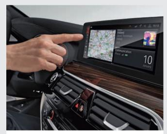
With **BMW Gesture Control**, certain functions can be operated by means of defined hand movements. For certain operations the system will, for example, recognise gestures such as 'swiping' or 'pointing' for accepting or rejecting an incoming call, or circular motions of the index finger to adjust volume.
