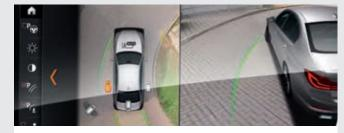
Parking Assistant with Surround View Camera makes parking and manoeuvring the vehicle easier. The Parking Assistant with linear guidance parks the vehicle automatically, parallel or perpendicular to the street. If the driver parks manually without the help of the Parking Assistant, Active Park Distance Control (PDC) offers additional protection against damage with the Lateral parking aid.
