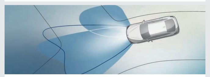
**LED Headlights with Adaptive headlights**, variable city and motorway light distribution and BMW Selective Beam provide optimum illumination of the road when driving in the dark. Even at a standstill, the integrated cornering lights are automatically activated by signalling or turning the steering wheel and are active at speeds of up to 35 km/h.
