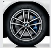
18" M light alloy Doublespoke style 662 M wheels, front 8J x 18 with 245/45 R18 tyres, rear 9J x 18 with 275/35 R18 tyres.
