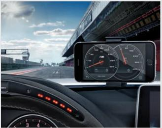
**BMW M Performance Drive Analyser.** The Drive Analyser comprises of an on-board diagnostics stick and a smartphone app to collect and analyse a variety of technical driving data.
