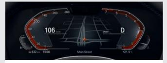
The newly designed **Instrument Display** with Black Panel technology and a screen diagonal of 31.2 cm (12.3") provides a highly impressive visualisation of the driving experience. The different modes and their specific displays – each of which has its own colour scheme and graphic style – can be displayed in the instrument cluster.
