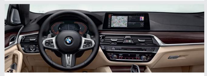
The newly developed interface design of **BMW Live Cockpit Professional with Navigation** makes using the infotainment system in the BMW 5 Series easier, more lucid and intuitive. The 26 cm (10.25") LCD display has Touch Functionality, configurable home screen, 3D Maps and can also be operated through iDrive Touch Controller, and Voice Control.
