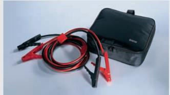
**BMW Jump Lead.** The copper cable jump lead is fully insulated with an integrated protective circuit and highly robust battery clamps. Delivered in a storage bag with two versions – 3.5 m long with a cross-section of 25 mm² or 4.5 m long with a cross-section of 35 mm² for vehicles with a large capacity.
