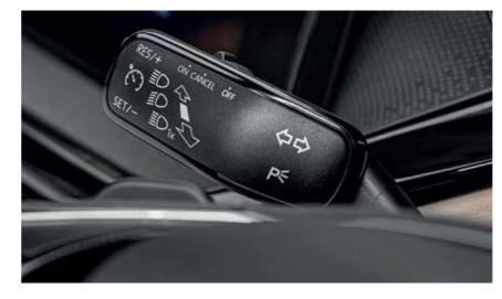
**CRUISE CONTROL** In addition to maintaining the preselected speed, cruise control enables you to increase or reduce speed without using pedals.
