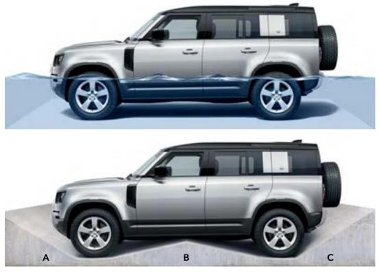
Ride Height Off-road<sup>†</sup> Standard A Approach Angle 37.5° 30.1° B Ramp Angle 28.0°<sup>++</sup> 22.0° C Departure Angle 40.0°<sup>++</sup> 37.7°
