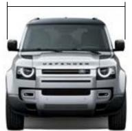
Front wheel track Air suspension 1 706 mm Coil suspension 1 704 mm
