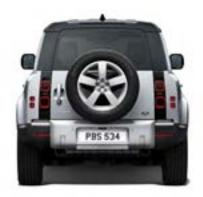
Rear wheel track Air suspension 1 702 mm Coil suspension 1 700 mm
