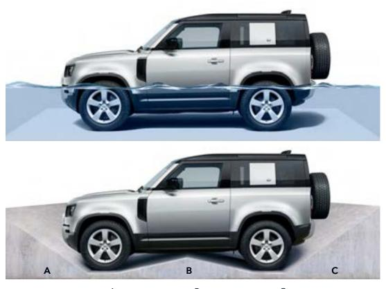
Ride Height Off-road\*\* - Coil (Air) Standard - Coil (Air) A Approach Angle 31.5° (37.5°) 31.0° (30.1°) B Ramp Angle 25.5° (31.0°) 25.0° (24.2°) С
